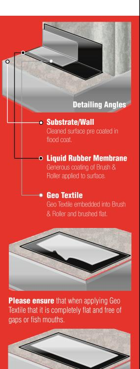
**The perfect finish for Geo Textile** leaves it flat to the surface and free of gaps fully embedded into the Brush & Roller below.
