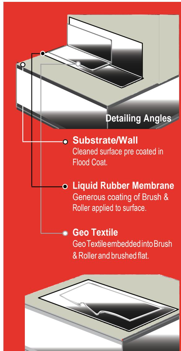
Please ensure that when applying Geo Textile that it is completely flat and free of gaps or fish mouths.
